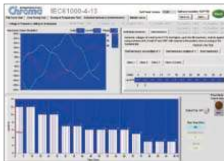
Voltage Harmonic & Interharmonic Test
